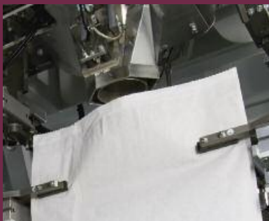
Dust-tight powder spout filling of products with high dust portions
