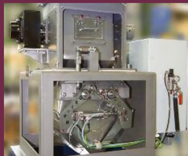
Net weigher dosing of granulated, grainy and lumpy products
