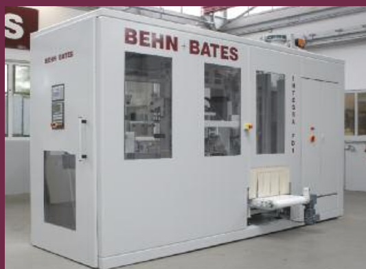
Expandable „Plug 'n Pack" designs INTEGRA FD and MINISEAL® with 1 to 3 filling spouts, output: up to 750 bags/h
