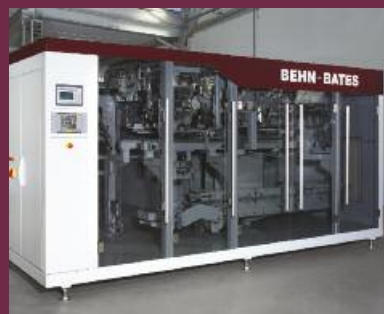
TOPLINE® fully automatic system with gross weigher for powders and net weigher for granules
