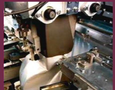
Flap spout filling of granulated, grainy and lumpy products
