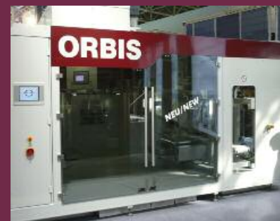
ORBIS® rotating system with 4 filling spouts especially for powders
