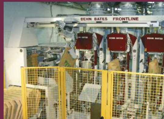
Fully automatic 1- to 3-spout installations with bag applicator and sealing stations, output: up to 750 bags/h
